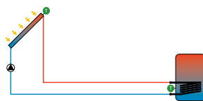
Internal heat exchanger, intelligent pump control
