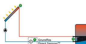
Internal heat exchanger, intelligent pump control
